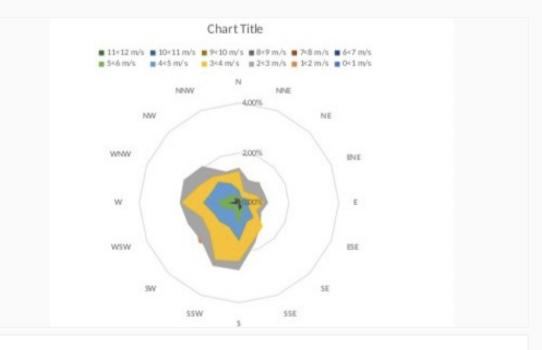
How the wind speed and its direction is distributed is visualized by a wind rose. Detailed data is compiled in the table. The wind direction is defined away from the origin e.g. if we liken the wind rose to a clock, a wind from south blows in the direction of midnight. The centered rings represents the percentage in time. For the simulations, four wind directions (S, SW, NW, W), were simulated and visualized with the dominant inflow wind speed 2.5 m/s (S, W, NW) and 1.5 M7s (SW).
